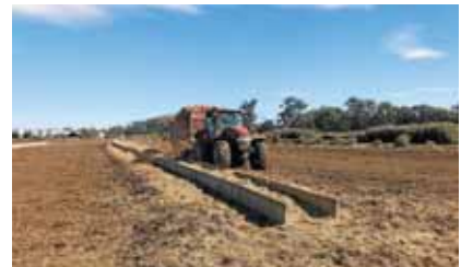
The feed wagon distributes the ration into the trough in the feedout area.
