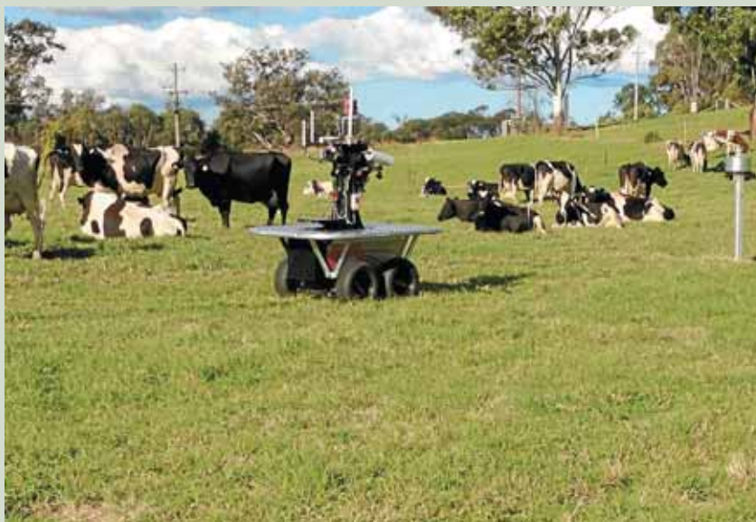
A prototype of the robotic herder being developed at the University of Sydney.
