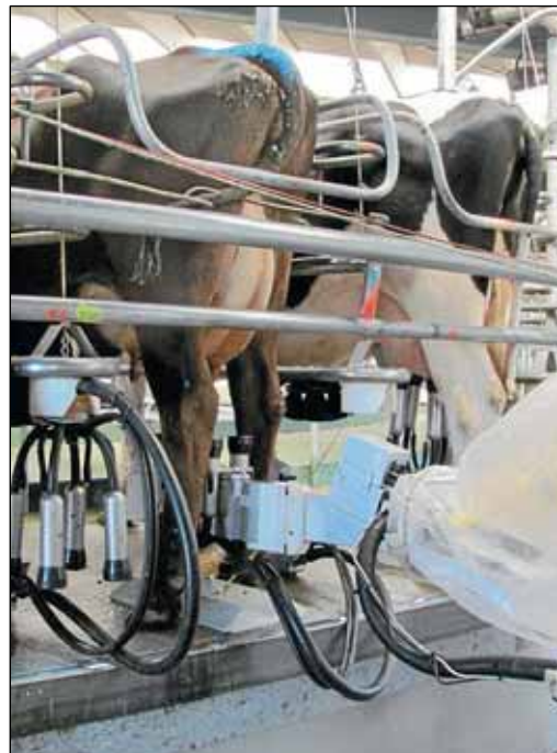
LEFT: With its hand upside-down, the robot grips the teat cups.
