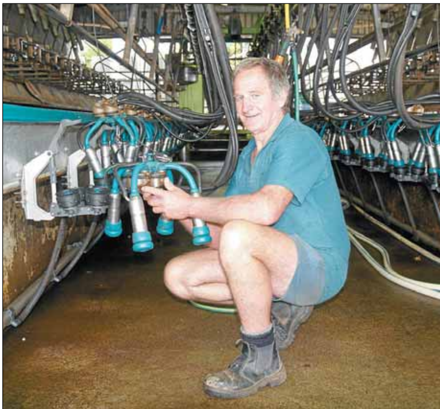
Rob Marshall with one of the WestfaliaSurge IQ clusters that he says have made milking faster.
