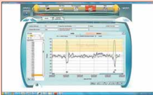
SCR Heatime removes false positives seen in activity-only heat detection, by looking for a corresponding drop in rumination.
