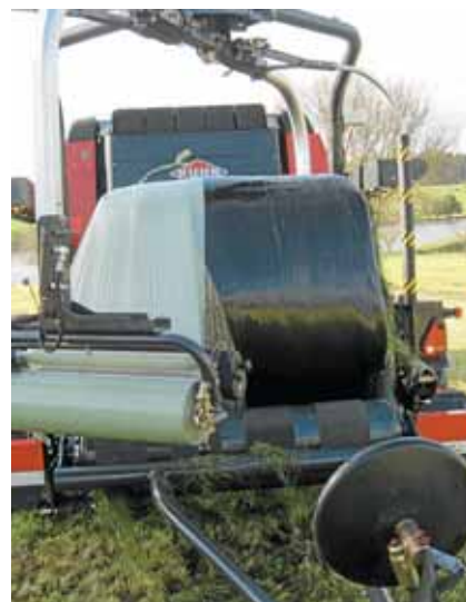
Figure 2: Stretch wrap film over netwrap on bale perimeter, before normal wrapping.
