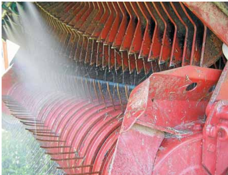
Figure 1: A liquid inoculant being sprayed from above and jetted from below.
