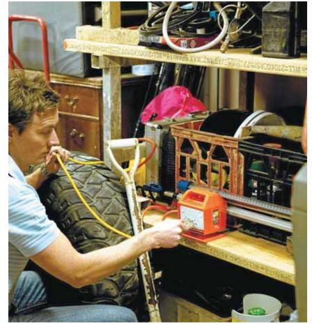
Good electrical practice: if electric extension leads are unavoidable, ensure they are connected to an RCD or safety switch.
