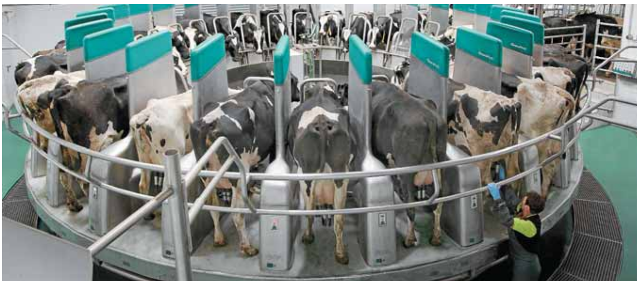
GEA's DairyProQ robot rotary milks cows three times a day on this German farm. Each individual milking stall module can also be switched to a manual mode, for example, to attach the teat cups by hand (see person in right of photo).
