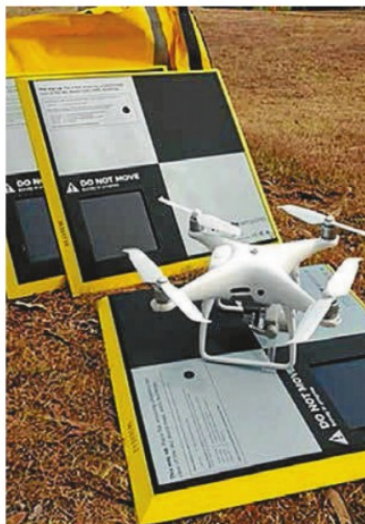
The drone with a high-resolution camera and ground control points with accurate GPS locations, which are necessary to accurately measure pasture height.
