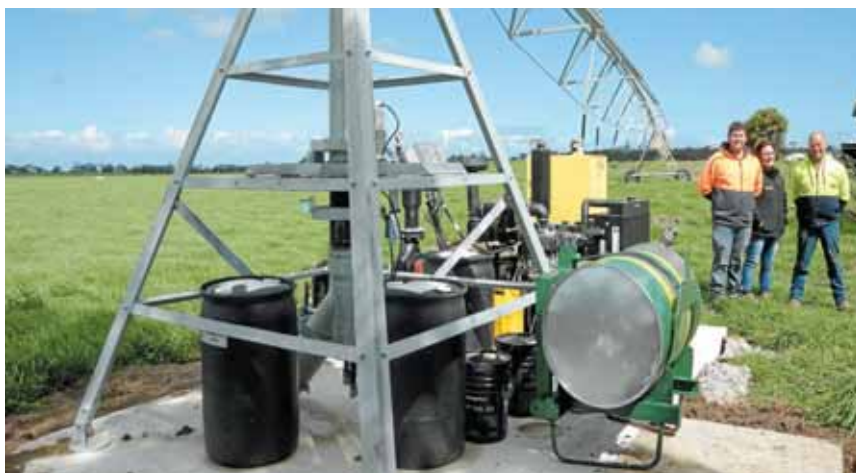
Terry, Clare and Trevor Porter at the head of the travelling irrigator, where the diesel pump, diesel engine and a temporary fuel tank have been installed on the concrete slab.
