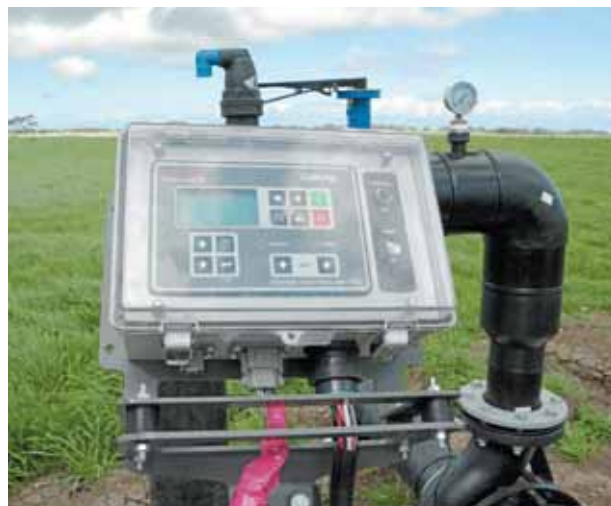
The control panel enables manual start up and automatic switch off of the irrigator and the pump. Photo by Jeanette Severs.
