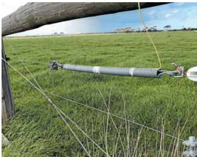
Pivot fence springs enable the 140-metre long irrigator to travel across the fences without impacting on wires or fence posts. Photo by Jeanette Severs.
