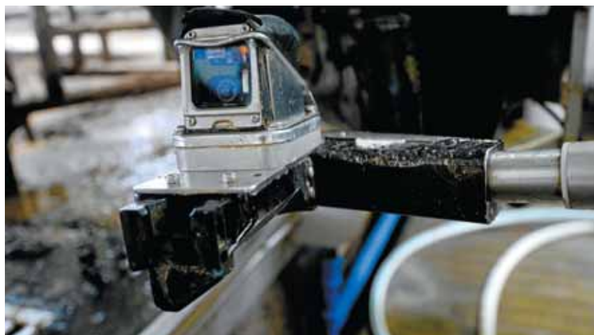
The camera helps guide the robot arm, and gets scrubbed clean automatically after each cow.
